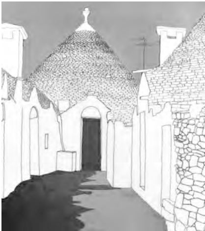
Fig. 18-20. Trulli at "water out", the drainage lines of the roof and the ground carry the water to a well or to an outdoor cistern to the house . This water serves the neighborhood (author: G. Mazzone)
